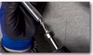
**3** Place the setting tool on the drill and set to hammer.
