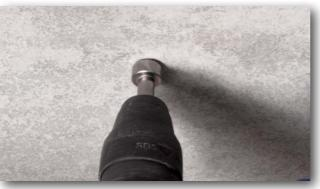
**2** The stop defines the optimum depth of the drill hole.
