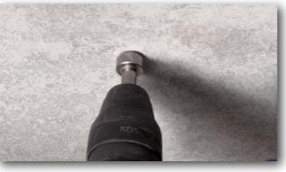
**2** The stop defines the optimum depth of the drill hole.
