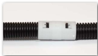
**3** Due to the transparency of the socket and the integrated stop point, the connection of the pipes can be checked.
