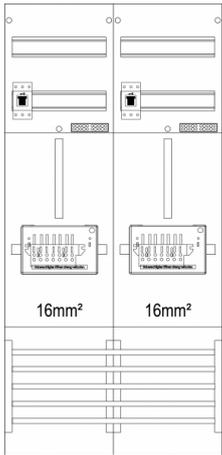
**Zählerfeld 2-feldrig, H=1050mm, 2-3.HZ 16mm<sup>2</sup>, 2 ZSK-Set, 2 HSS, Z21B-16-ZSK-HSS**
